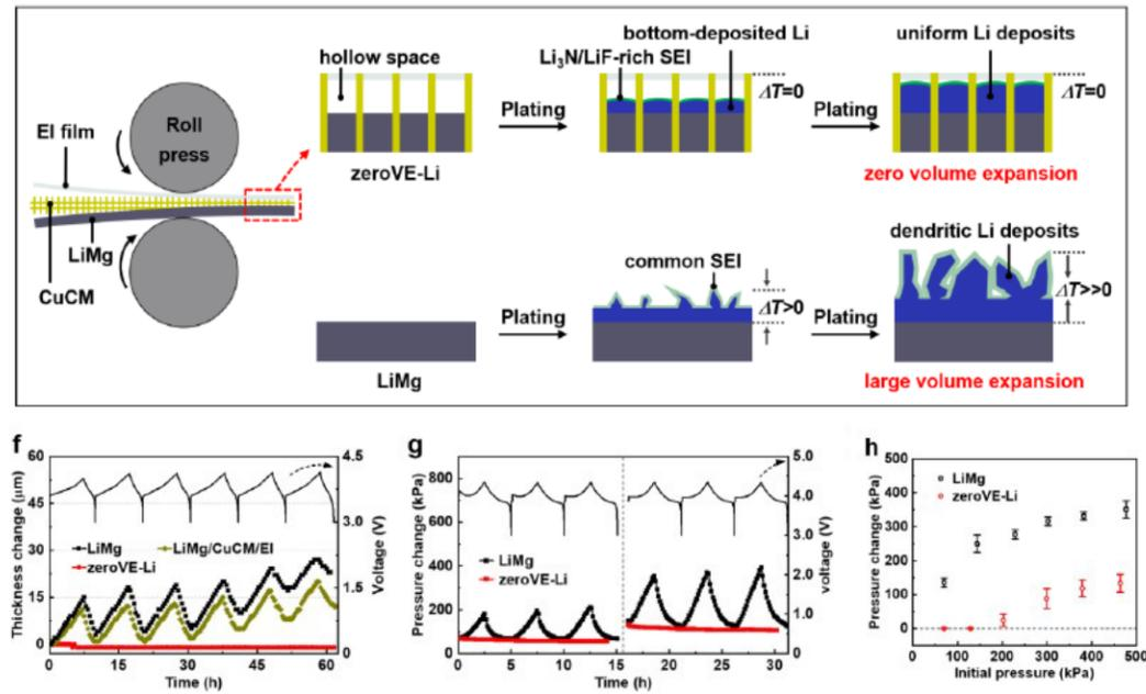
**Conclusion:** The modified lithium metal anode can significantly reduce the volume expansion of the cycle process.
