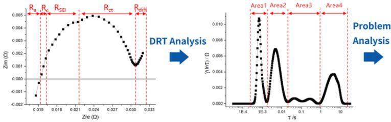
**Contact impedance  $R_{\Omega}$**  : The sum of all electronic resistances inside the battery, which is related to various problems
