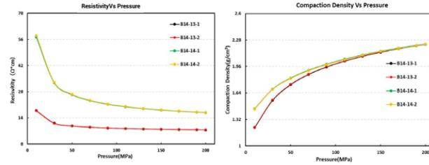
**Conclusion 1:** The conductivity of B14-13 is superior to that of B14-14. This is primarily due to its lower porosity, which enhances particle contact throughout the compression process, resulting in better conductivity.
