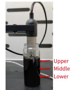
On the first and fourth day of testing, the resistivity of the upper and middle channels increased, while the resistivity of the lower channel decreased, indicating that after four days of shelving, the slurry shows obvious settlement.
