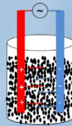
$$\text{Resistivity } (\Omega \cdot \text{cm}): \rho_e = \frac{U}{I} \times \frac{S}{l}$$
