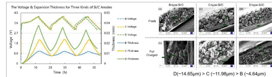
**Test Conditions:** ☑ NCM/Si/C Coin Cells ☑ Si/C#D(~14.65um) ☑ Si/C#C (~11.98um) ☑ Si/C#B(~4.64um)
