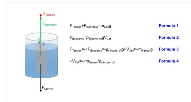
By combining Newton's law (formula 1) and Archimedes' buoyancy principle (formula 2), specialized sensors are used to measure the real-time mass changes of the cell during the charge & discharge process, and then the cell's volume changes can be further calculated (formula 3 and 4).
