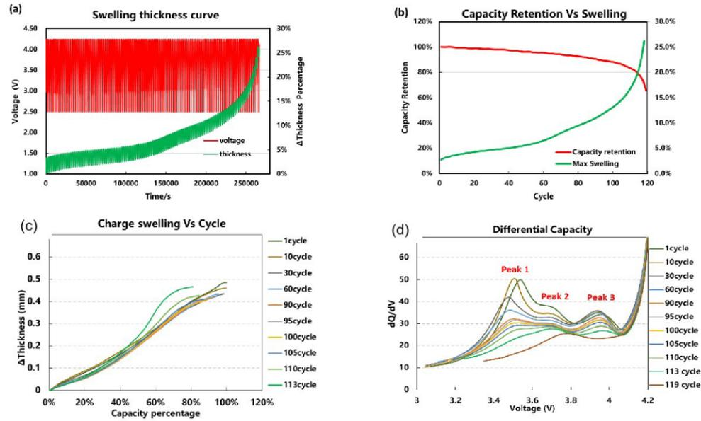
**Test Conditions:**  NCM811-Gr Prismatic Cell (50 Ah)  Voltage: 3V ~ 4.2V  Rate: 1C
