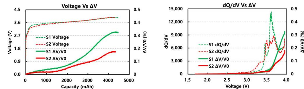
21700 Cell parameters: Sample 1-15%SiC ; Sample 2-10%SiC
