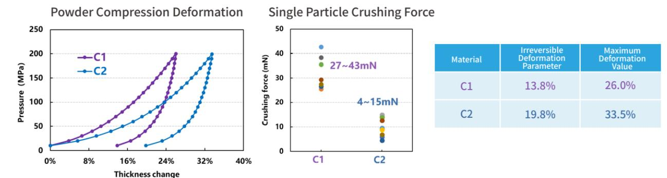
**Conclusion:** The compressive property of particle C1 is stronger. Hence, C1 powder shows a higher compression modulus than that of C2.
