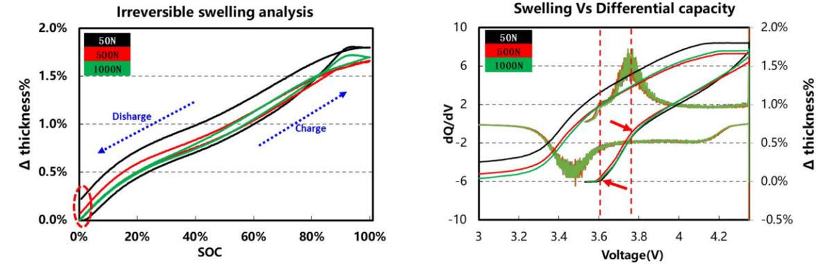
**Test Conditions:**  NCM523/Gr Prismatic Cells(2400 mAh)  34cm\*46cm\*106cm(T\*W\*L)  Pre-stress: 50N/500N/1000N
