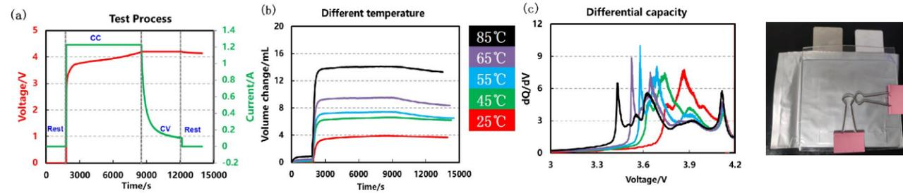
**Test Conditions:** ☑ NCM/Gr Pouch Cell ☑ Rate: 0.5C ☑ Charging: CC 4.2V ☑ Capacity: 2400mAh
