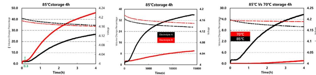
**Test Conditions:** ☑ 4.2V fully charged ☑ storage at 85°C for 4h
