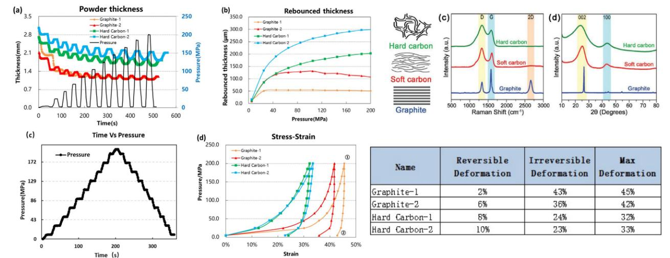
**Conclusion:** the conductivity of graphite is greater than that of hard carbon, so is its powder compressibility.
