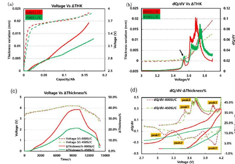
**Test Conditions:** ☑ Pouch Cell(stacking) ☑ 200 mAh (1 cycle) ☑ Cathode: NCM811
