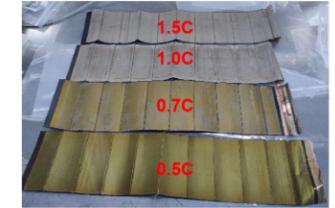
**Test method:** Charge the cells at different rates and discharge them at the same rate to analyze the differences in their voltage curves and swelling thickness curves.
