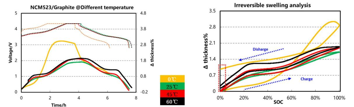
**Test Conditions:**  NCM523/Gr Prismatic Cells(2400 mAh)  34cm\*46cm\*106cm(T\*W\*L)
